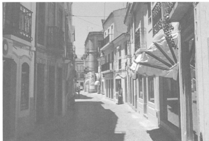
Fig. 5. Street scene in Portugal illustrates design responses to variable climatic conditions, overhands and shaded balconies, adjustable awnings, ventilating shutters, bright and light colors.
